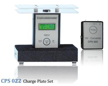
To test air ionization systems by measure the discharge time
